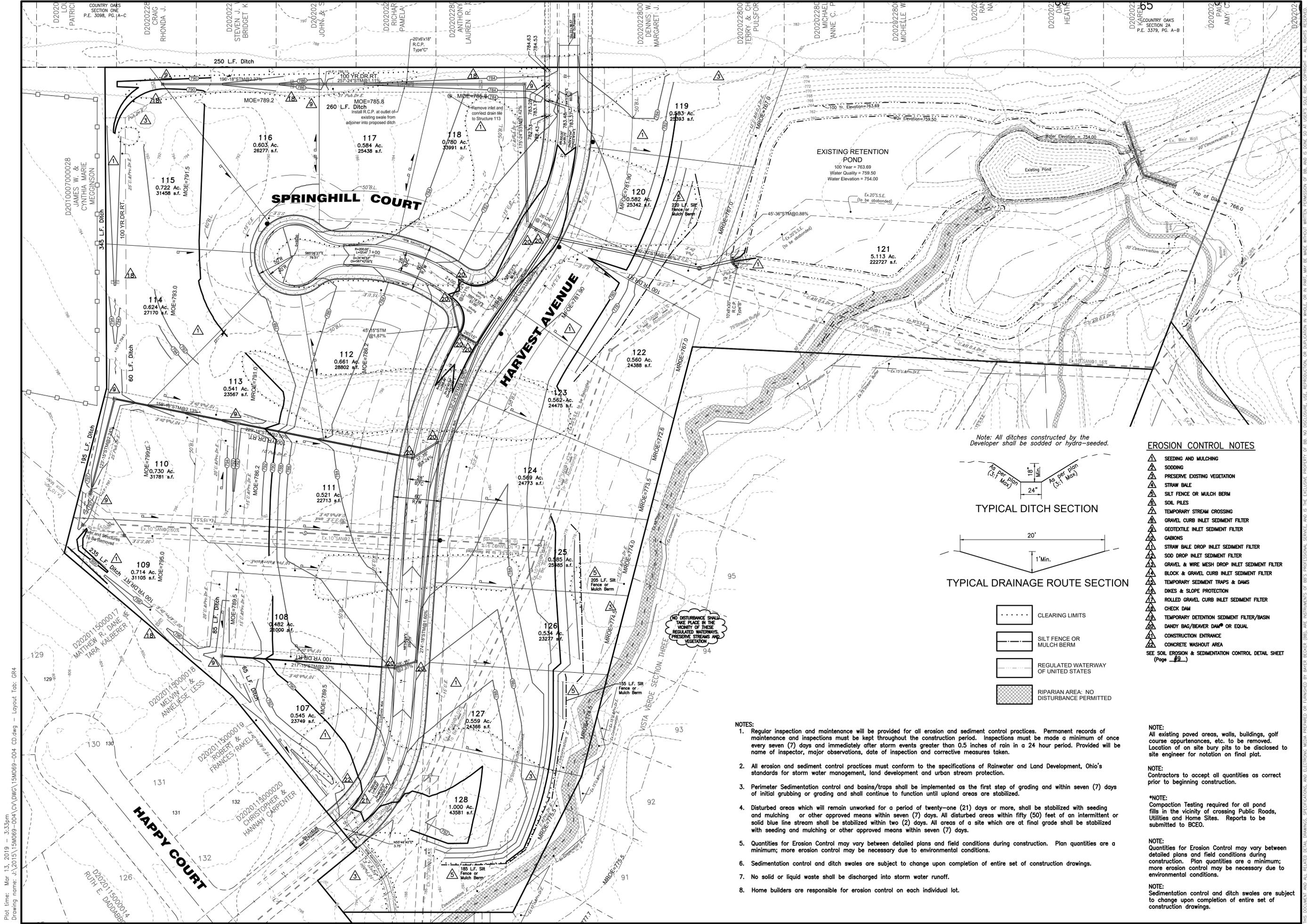
Note: All ditches constructed by the Developer shall be sodded or hydra-seeded.
