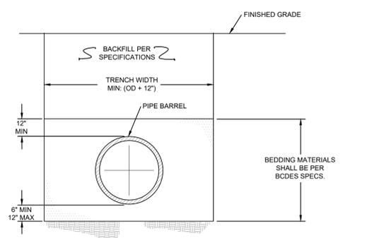
TYPICAL TRENCH DETAIL WATER MAIN INSTALLATION
