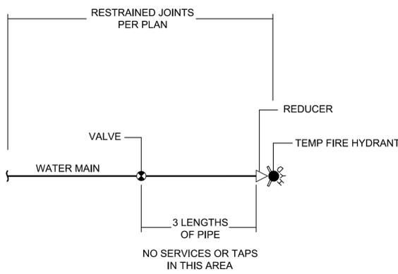
DEAD END DETAIL WITH TEMPORARY FIRE HYDRANT
