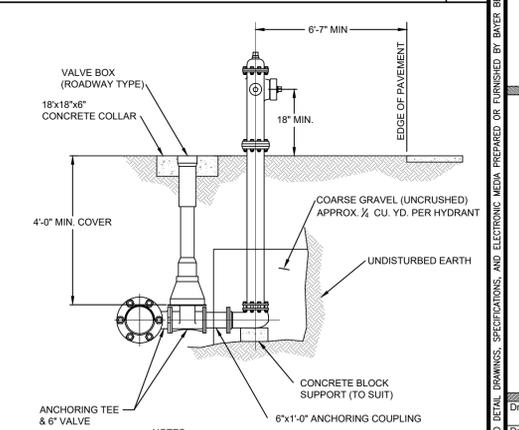
TYPICAL FIRE HYDRANT INSTALLATION
