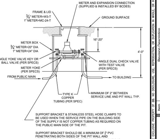
STANDARD INSTALLATION FOR 3/4" AND 1" WATER METER SETTINGS
