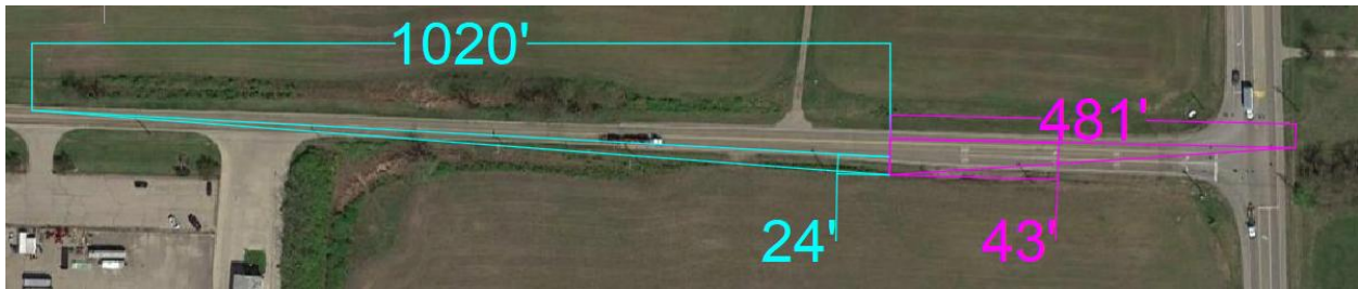
Figure 7.1a: “Development Exit” Sight Triangle
