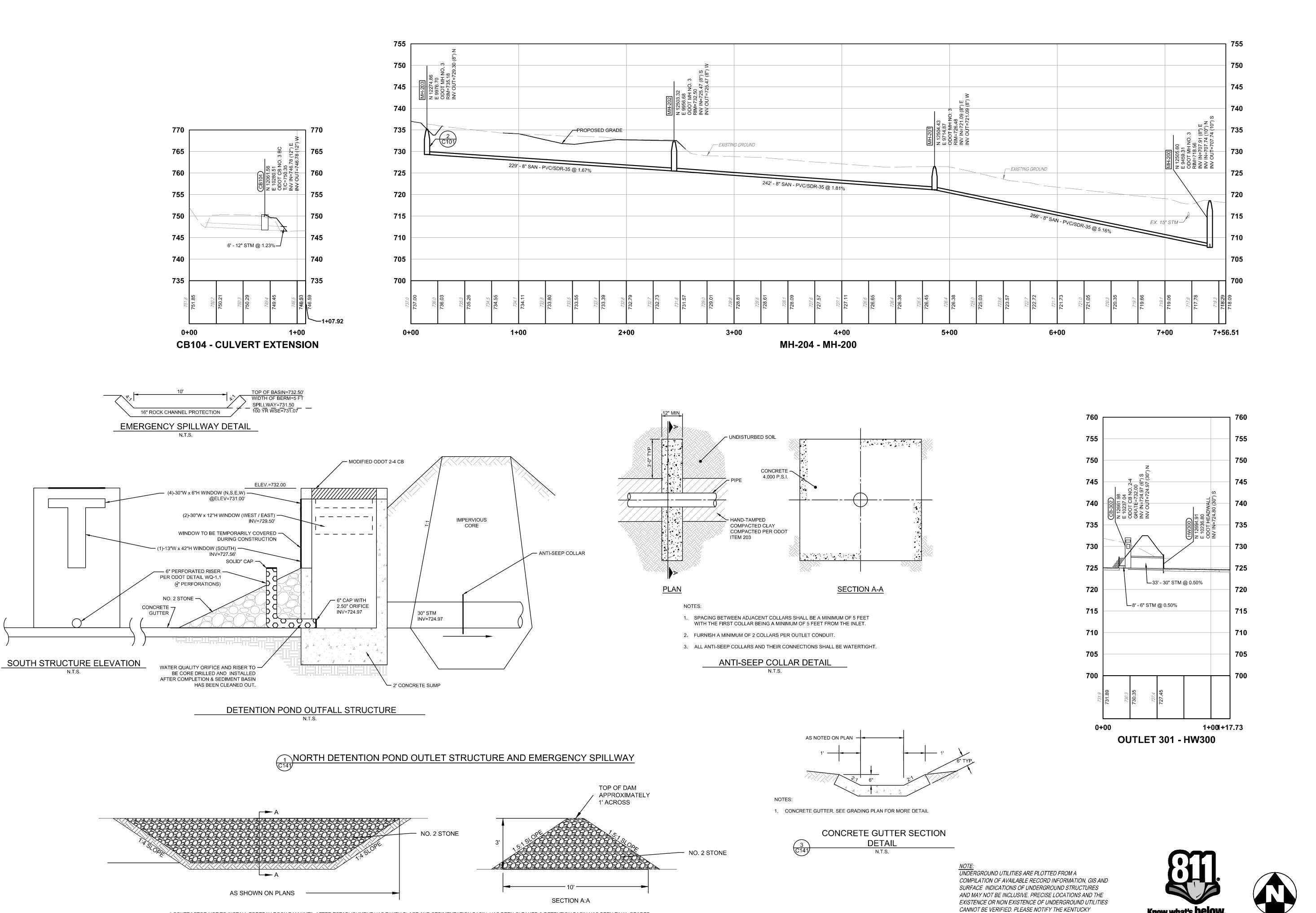
\* CONTRACTOR NOT TO INSTALL FOREBAY ROCK DAM UNTIL AFTER ESTABLISHMENT HAS TAKEN PLACE AND SEDIMENTATION BASIN HAS BEEN CLEANED & DETENTION BASIN HAS BEEN FINAL GRADED.
