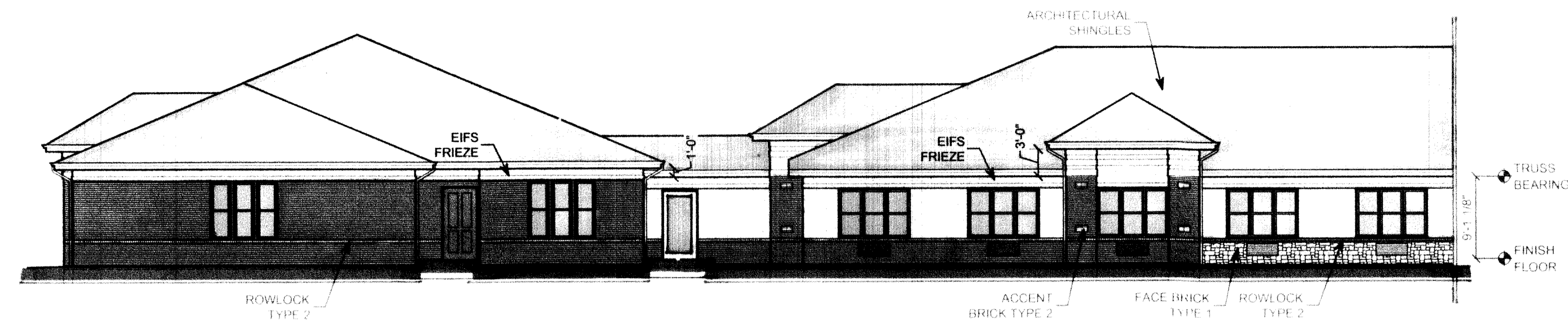
PARTIAL EAST EXTERIOR ELEVATION (C)
