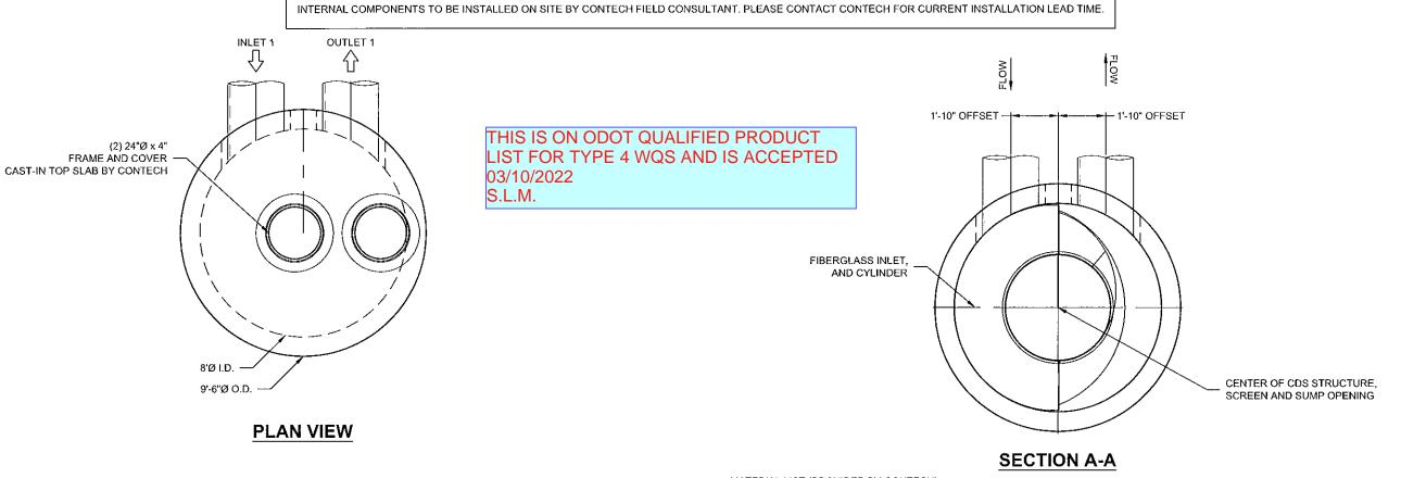
CONTECH TO CAST-IN FRAME AND COVER **FIBERGLASS** SEPARATION CYLINDER & INLET RIM ELEV. = 660.48 ± OUTLET 1 TOP OF STRUCTURE INLET 1 ELEV. = 660.47 24"Ø HDPE 24"Ø HDPE (32"Ø OPENING) (32"Ø OPENING) INLET PIPE 1 INV. ELEV. = 656.56 OUTLET PIPE 1 INV. ELEV. = 656.56 PERMANENT POOL ELEV. OIL BAFFLE SEPARATION **SCREEN** SOLIDS STORAGE SUMF OUTSIDE BOTTOM 10 M ELEV. 646.56 - 9'-6"Ø -
